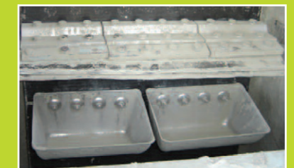
Braime Clamp Belt Splice on 4B Steel Web Core Belt
