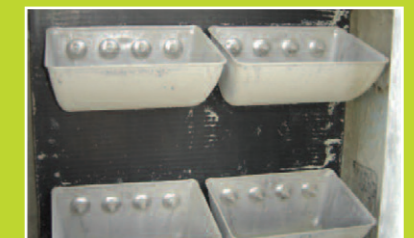
Starco Jumbo Buckets on 4B Steel Web Core Belt Cement Application
