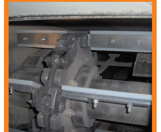
UHMW Paddles on "T" Plate Flights - Drive End
