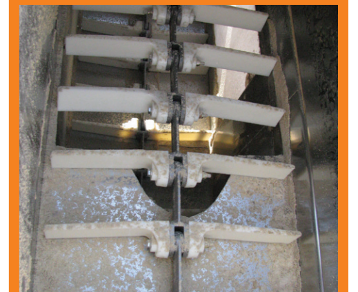
Feed Mill Application using Bolt 'N' Go Chain with Nylon Flights
