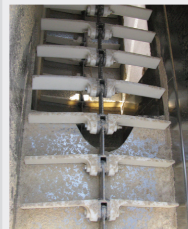
Feed Mill Application using Bolt 'N' Go Chain with Nylon Flights
