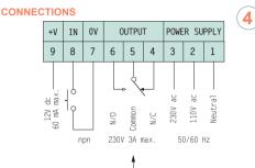
Note: Relay energises above or below 'Trip Level' setting. See overleaf for programming details.
