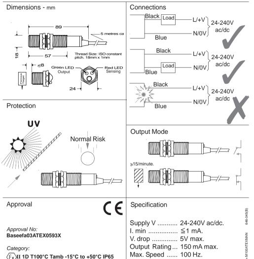
**Note!** If long cable runs are to be used, the wiring should **not** be positioned adjacent to cables carrying high voltage or current.
