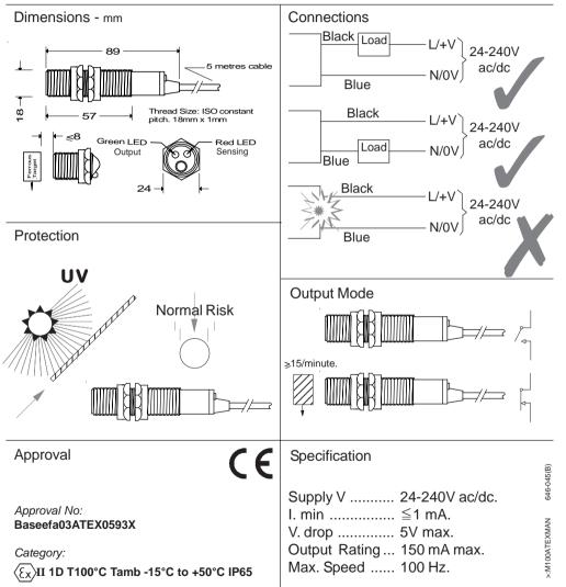
**Note!** If long cable runs are to be used, the wiring should **not** be positioned adjacent to cables carrying high voltage or current.
