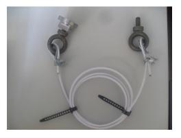
For rip detection two Bulldog units are required one at either side of the conveyor, the BRW belt rip wire connects the two units together by magnetic attachments at each Bulldog. The belt rip wire is placed on the underside of the conveyor approx 25mm down from the bottom of the belt see the figure below.
