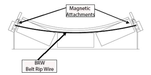
The length of the BRW Belt Rip Wire can be adjusted to suit the width of the conveyor by loosening the steel wire clamp and adjusting the cable length through the eyebolt as shown in fthe figure below.
