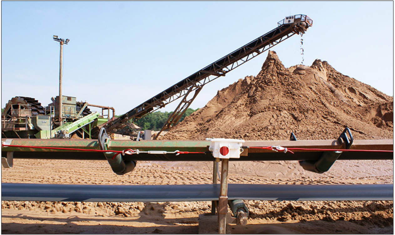
Pullswitch Installed on Open Conveyor at Sand and Gravel Facility
