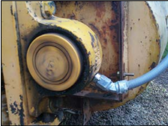
WDB20V3C bearing temperature sensor shown installed on a tail bearing of an enclosed belt conveyor.
