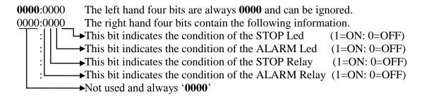
When a relay is considered to be 'ON' we mean energized and when 'OFF' we mean deenergized.
