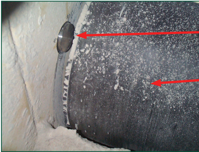
Touchswitch™ Installed at Drive End of Enclosed Belt Conveyor (Inside View)
