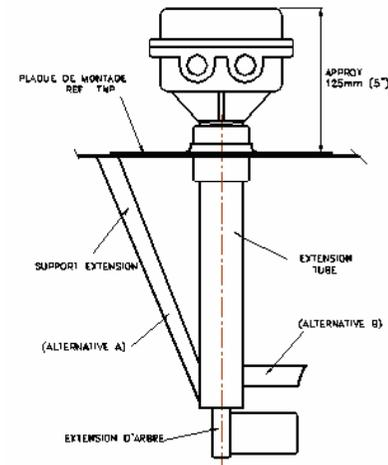
LES EXTENSIONS D'ARBRE ET TUBE DE PROTECTION PEUVENT ÊTRE FOURNIS POUR UN NIVEAU BAS OU HAUT. LE RULI EST MONTÉ SUR LE TÔIT DU SILOS OU SUR LA TREMIE.
