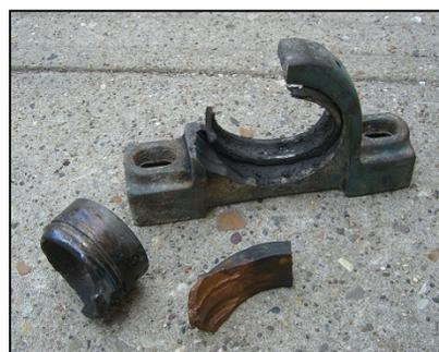
**Example of Bearing Failure**
