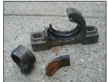
Example of Bearing Failure
