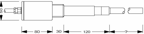
Standard probe ATPP( polypropylene) and ATPK ( peak )
