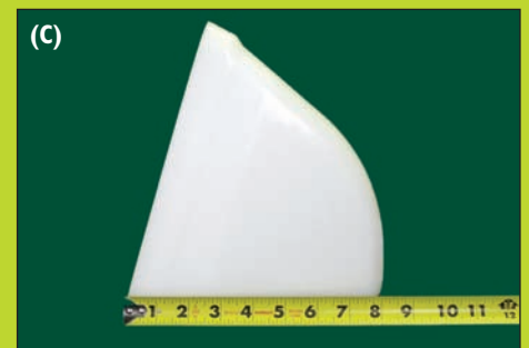
(C) With elevator bucket back laid flat, measure back height (C). Con la espalda del cangilón plano, medir la profundidad (C).
