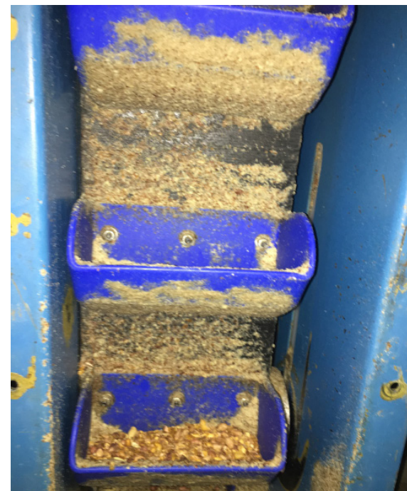
Peanut Build-Up Inside Buckets
