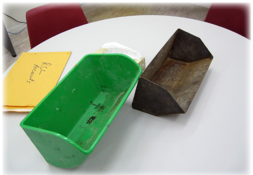
Image 2: Old Style Fabricated Steel Bucket & CC type bucket
