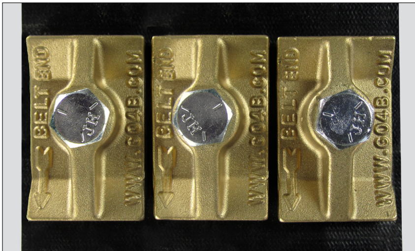
Top View of Vise Splice Installation
