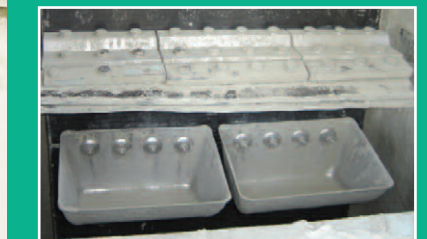
Braime Clamp Belt Splice on 4B Steel Web Core Belt
