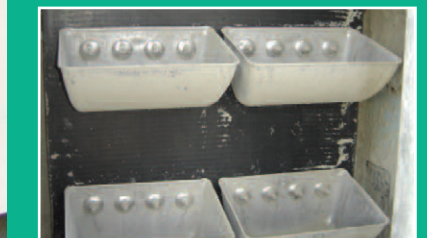
Starco Jumbo Buckets on 4B Steel Web Core Belt Cement Application
