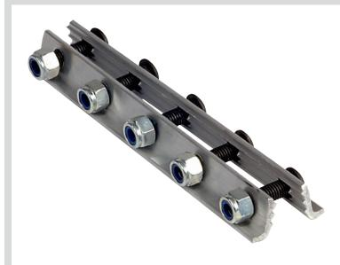
The **Gripwell** light duty aluminum fastener secures belting on bucket elevators. The two ends of the belt are gripped between extruded serrated plates, clamped together by zinc plated high tensile bolts, safely secured by plated self-locking nuts to give a strong reliable and rustproof fastener.
