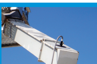
Binswitch Installed on Bucket Elevator Spouting (with SMP, BAS & conduit adapter)
