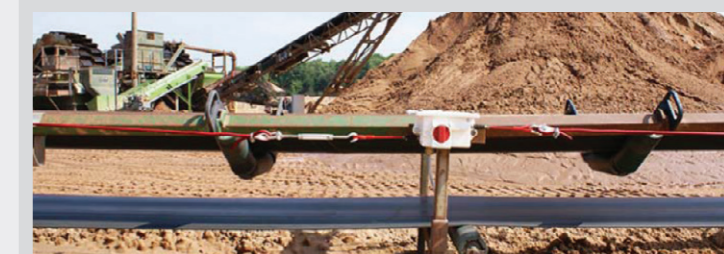
Pullswitch installed on open belt conveyor
